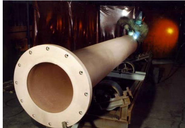
An electro-slag melting crucible for high temperature alloys from Zak Inc
