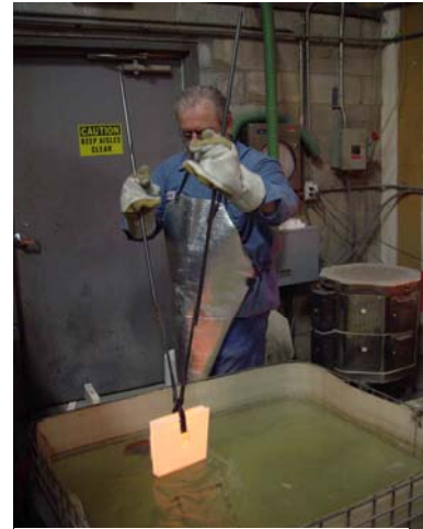
Testing ceramics for thermal shock at Blasch Precision Ceramics
