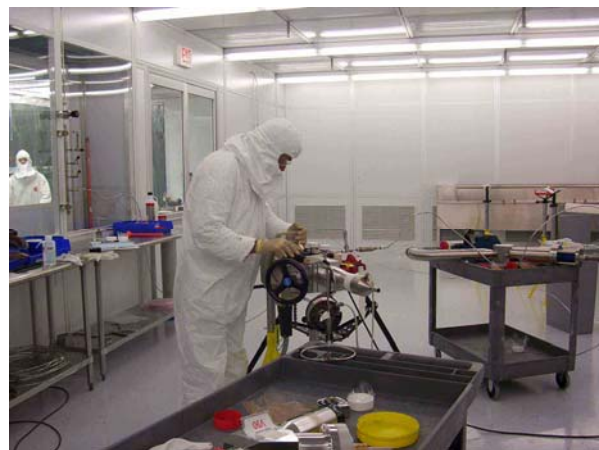
Orbital welding stainless steel tubing for a high purity gas delivery system by a TFS technician
